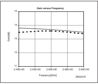
Figure 14. Gain vs. frequency
